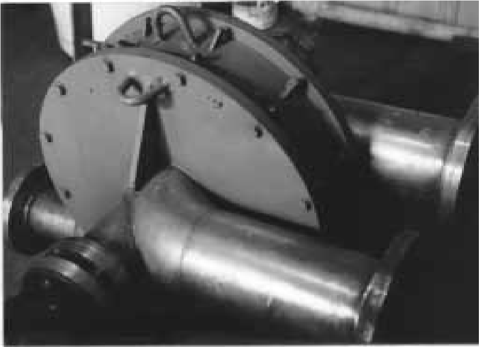
Salt Brine Geothermal Turbine
