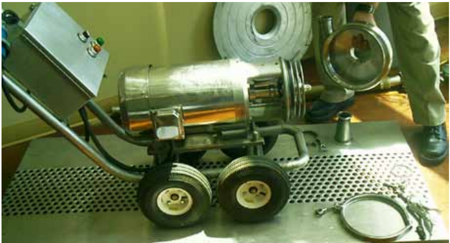
Sanitary Tesla Pump used by Tesla Engine Member Frey Organic & Biodynamic Wines. Used to avoid the sheering effects that damages conventionally pumped wines
