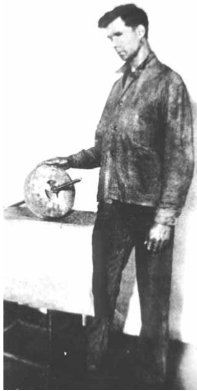
The Runner of the 110 Horsepower Engine Measures 9 \frac{3}{4} " in diameter and Weighs Twenty Pounds.
